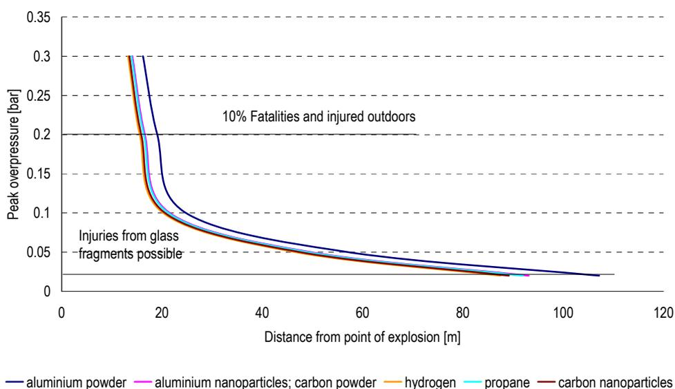
As shown in Fig. 4, the curves for all substances compared lie very close. In the present case of a 20 m<sup>3</sup> vessel, fatalities must be anticipated up to a distance of approx. 20 m from the point of explosion, should persons be present within this distance. Injuries from glass fragments are possible up to a distance of approx. 90 m.
